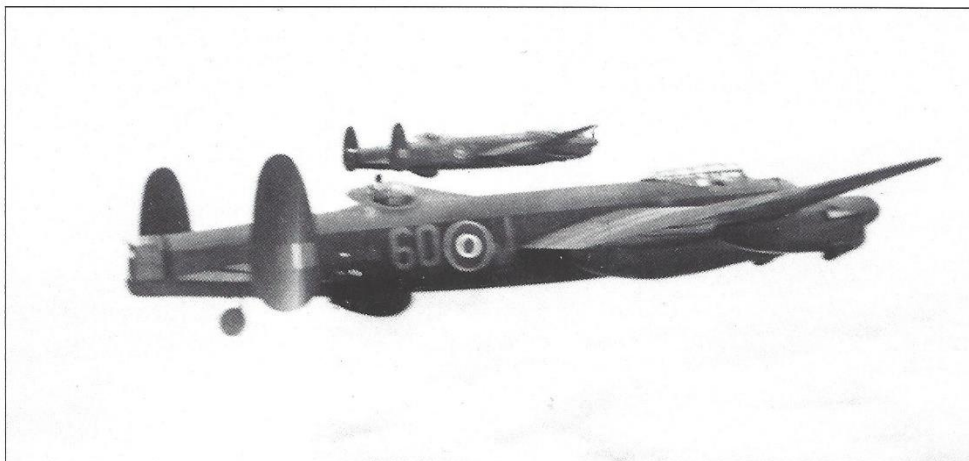
Above: 60-J and 60-Z heading out on a bombing mission. Note the open radiators on the nearest aircraft, an unusual sight on Lancasters at height.
