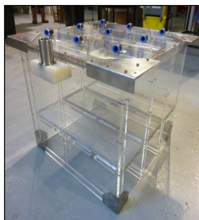
Fig. 10 Side view of the 3-Chamber-Box Scrubber (without Dixon rings).
